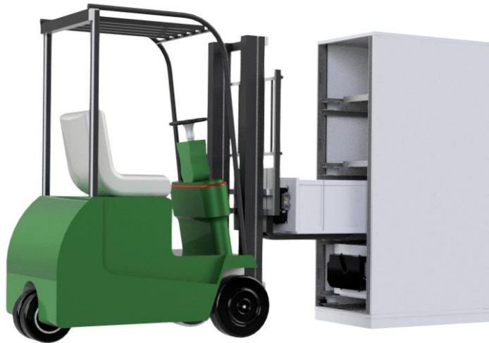
Figure 36 – battery moved with forklift truck
