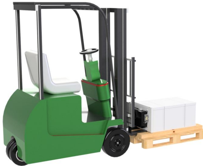
Figure 19 - Inserting the forklift between wooden beams to lift the battery from the pallet.
