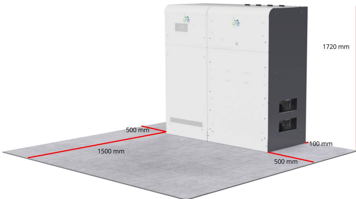
Figure 23 – Minimum distances of UNE ZHERO S10 for Battery Box and Inverter Box
